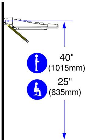
This mounting height is a recommendation for an ergonomic workstation. If user elbow heights are different than this, you should change mounting height to accommodate user elbow heights. (Change mounting height one inch for every one inch difference in user elbow heights).
