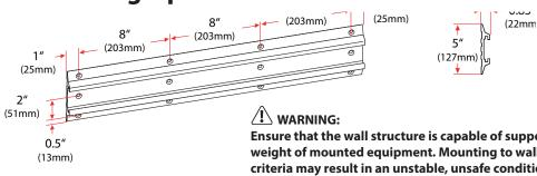
Ensure that the wall structure is capable of supporting four times the total weight of mounted equipment. Mounting to wall surfaces that do not meet this criteria may result in an unstable, unsafe condition which could lead to personal injury and/or property damage. Consult a construction professional if you have any doubt about what this means in regard to your particular application.
